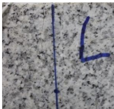
(a) BSG-THB01 左端面裂纹
